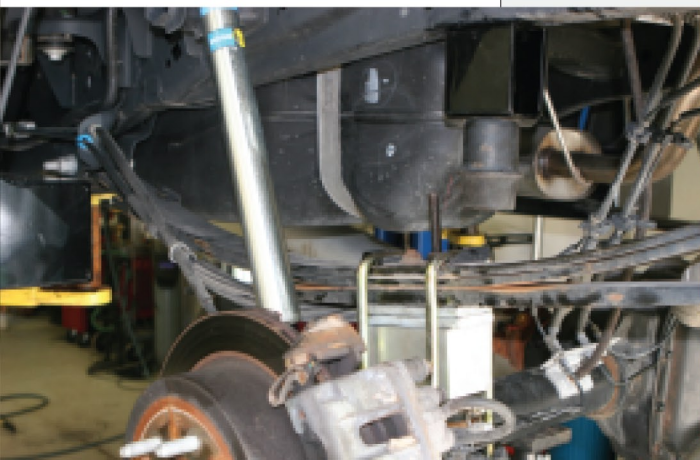
▼ Rear lift with new Bilstein shock.
