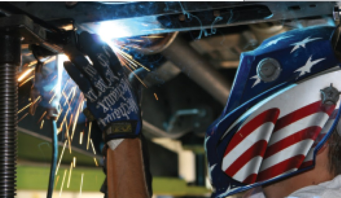
▲ Eric from FabStuff MIG welding SUPERLIFT bracket.
