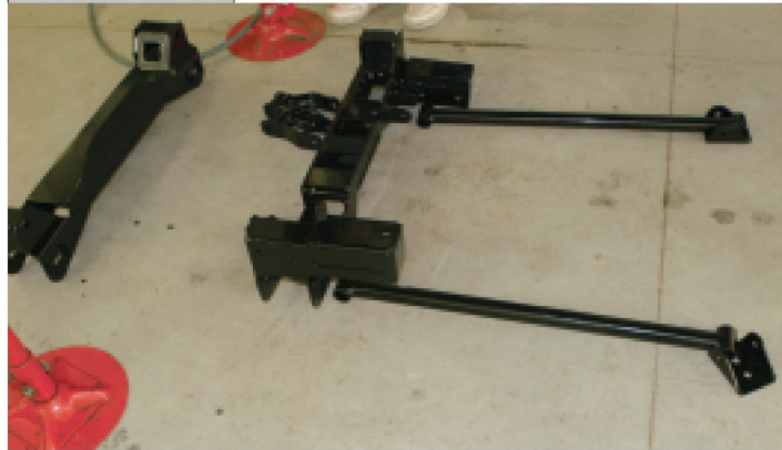
▲ Some of the core Superlift components. ▼ Stock steering knuckle compared to Superlift's knuckle.
