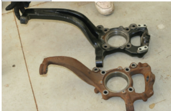
▲ Some of the core Superlift components. ▼ Stock steering knuckle compared to Superlift's knuckle.
