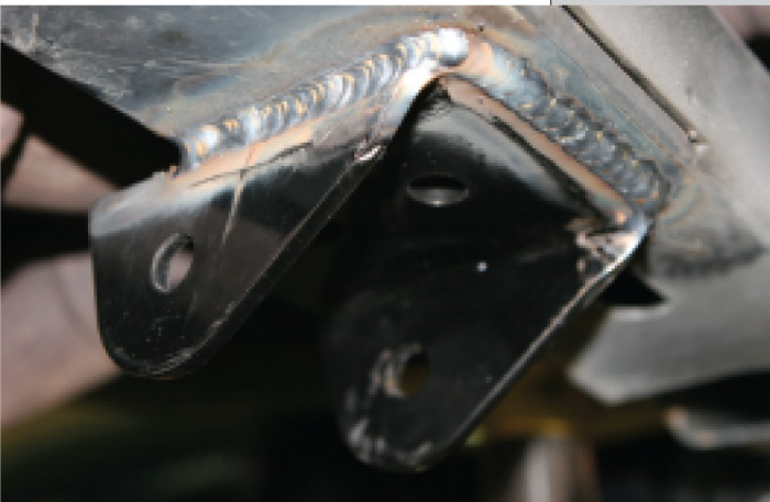
▲ Eric from FabStuff MIG welding SUPERLIFT bracket.
